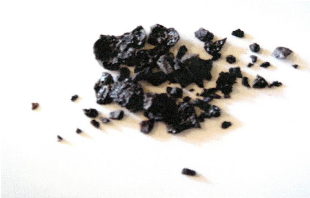
**Photograph 15: LWA Produced from fired briquettes after crushing and sizing**
