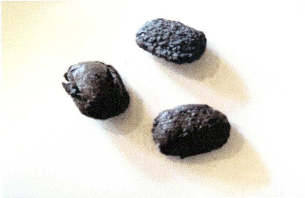
**Photograph 17: Bloated 20 cc Briquettes after Firing at 2200° F**
