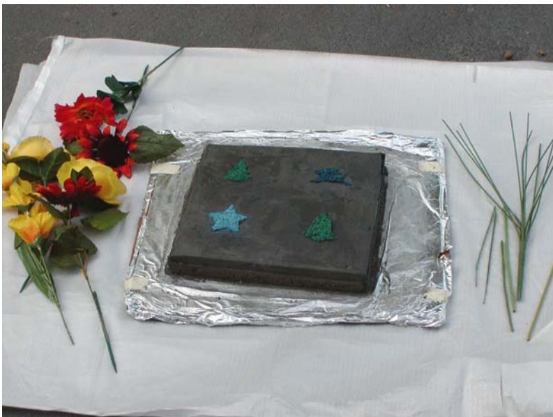
Above and Right: Fly ash and feldspar stepping stones reinforced with plastic coated scrap wire (flower stems)
